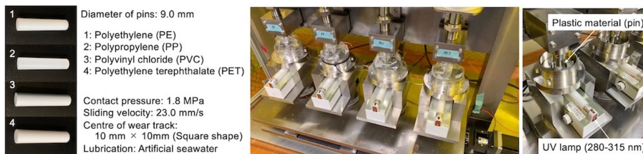
Fig. 1 Pin-on-disc machine for production of microplastics.
