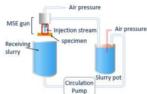
Fig.2 Schematic diagram of MSE apparatus
