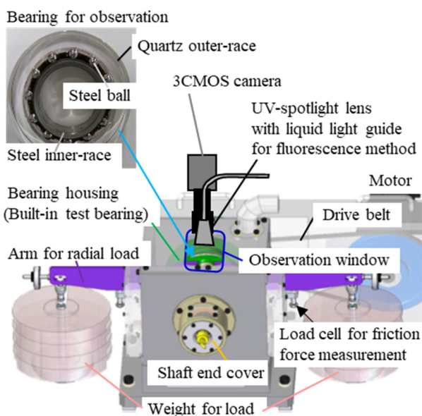
Fig. 1 Outline illustration of test apparatus (Optical systems are for fluorescence method)
