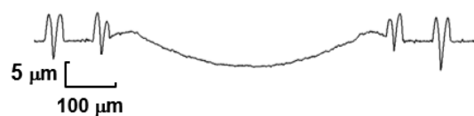
Fig. 8 Surface profile of wear scar of the textured aluminum alloy disk (SA162) when low friction generates.
