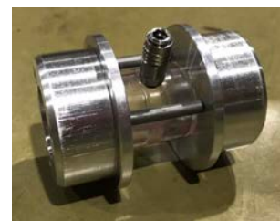
Fig. 3 Cartridge-type test bearing
