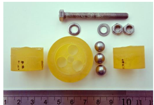
Fig. 1 Parts used in a synchronized phase transmission for 1:4 reduction
