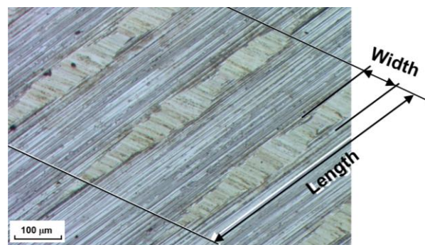
Fig. 5 Representative wear scar of the disk with streak, and definition of “wear width and length” of the disk.
