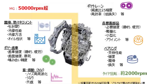
Fig.6-2 Effects on Transmission elements due to higher RPM
