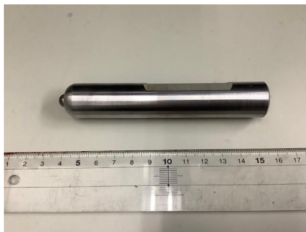
Fig. 1 Appearance of FSSW tool prepared in this study. The tip on the left side is the developed cermet material.
