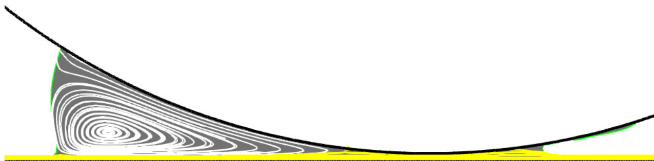
Fig. 3 Enlarged view of oil film profile with streamline in vase with zero gravity
