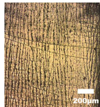
Fig. 3 OM image of Ag-DLC after tape bending test
