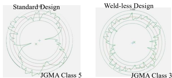
Fig. 4 JGMA/JSA tolerance classification on cylindrical
