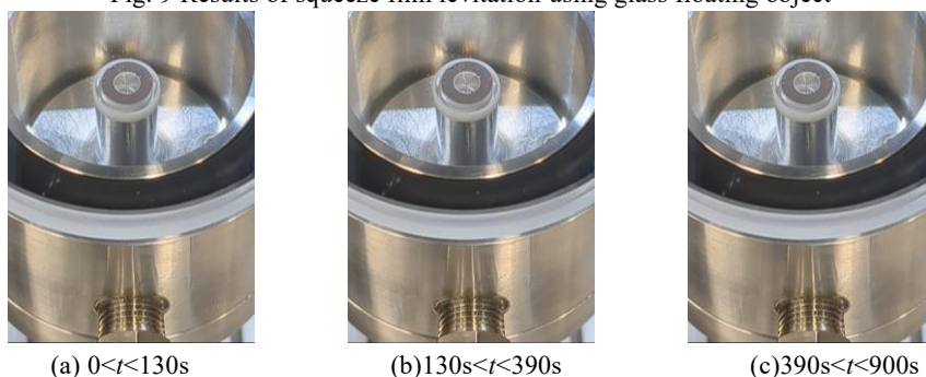
Fig. 10 Diffusion pump oil behavior at each time
