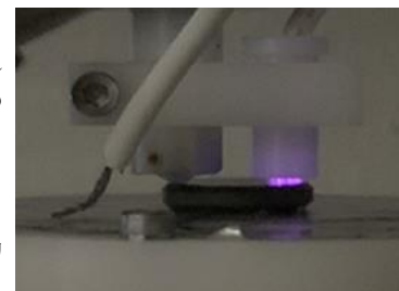
Fig.2 DBD persists in the gap between the glass plate and the a-C:H coated disk
