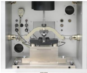
Fig.1 Sliding testing machine
