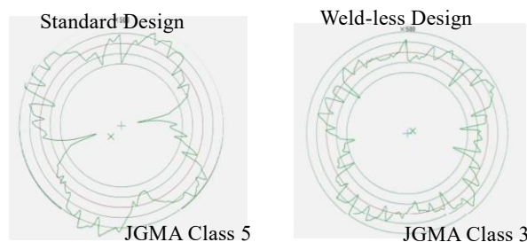
Fig. 4 JGMA/JSA tolerance classification on cylindrical
