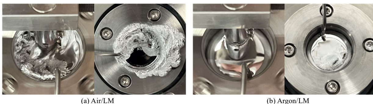
Fig. 3 Comparison in liquid metal conditions during and after tests with liquid metal lubrication in air (a) and argon (b)
