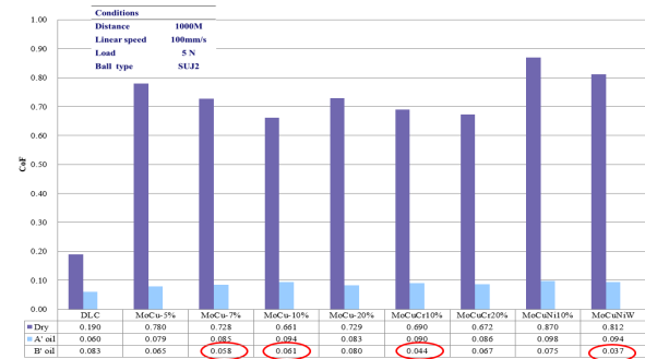
Fig 3. Friction coefficients of various Mo-Cu-X-N systems
