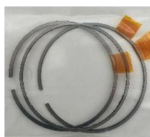
Fig.7 Combustion chamber parts exposed to hydrogen gas, such as pistons and piston rings used in hydrogen engines
