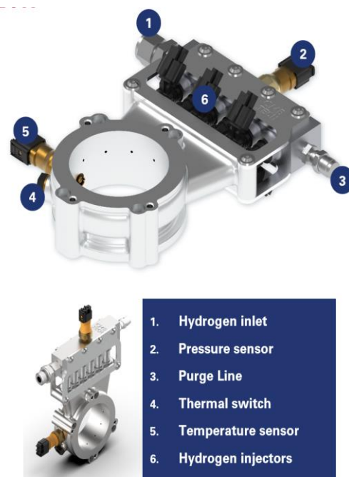
Fig 4 H2 dual fuel – Injection manifold
