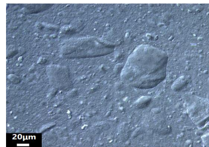
Fig. 1 DIC optical microscope image of the sample used in this experiment (thickness: 20 \mu m as the spacer)
