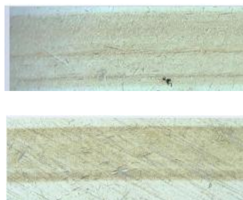
Fig. 6 Observation of ball surfaces, No voltage charge (Top), voltage charge (bottom)
