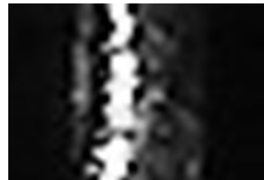
Fig. 5 Speckle patterns with parallel and perpendicular surface roughness (46×32 pix)
