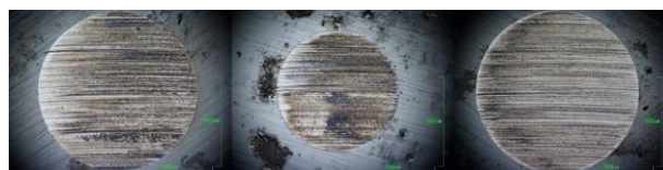
Fig. 4 Wear scar on the pins constant load test. From left to right: test results for H 2 , air and Ar conditions.
