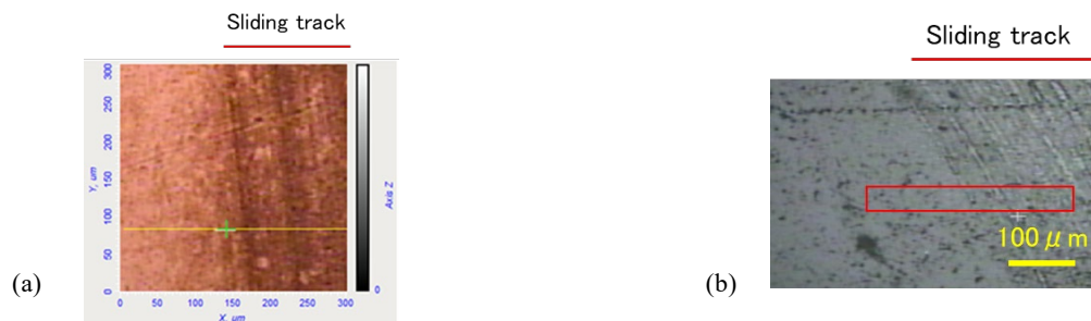
Fig.4 Optical image of sliding track on (a) ESB resin and (b) SBR
