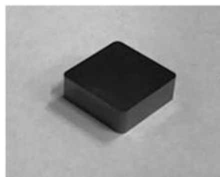
Fig. 3 Appearance of the \text{Ti(C, N)}-(\text{Ti, W})(\text{C, N})-\text{W} cermet cutting tool prepared in this study 3) .
