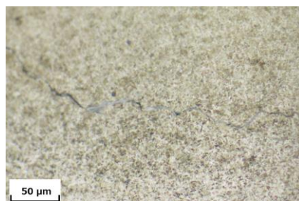
Fig. 4 Cross-sectional image of the interior of Damage of PAO2
