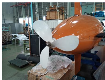
Fig. 2 A thruster on an underwater drone.
