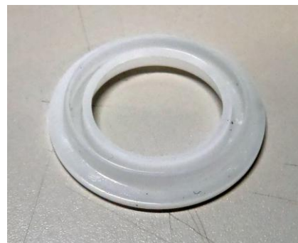
Fig. 3 The prototype POM shaft seal.
