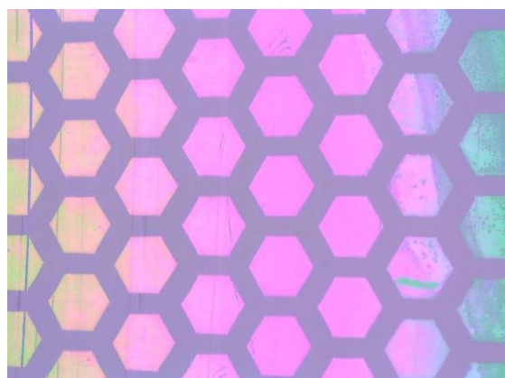
Fig. 9 Surface image on hexagon pillar texture, 0.2 MPa, 40°C, 32 mm/s
