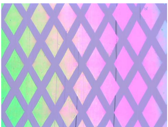
Fig. 11 Surface image on rhombus pillar texture, 0.2 MPa, 40°C, 32 mm/s
