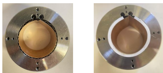
(a) Bump foil (b) Viscoelastic foil
