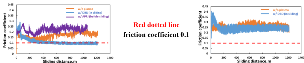
Fig. 3. Friction coefficients according to obtained for a-C:H disk against \text{Si}_3\text{N}_4 ball (left) or SUJ2 ball (right).
