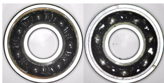
(a) Crown-shaped resin cage (b) Corrugated cage
