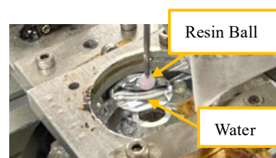
Fig.2 Image of the test stage during water-lubricated testing
