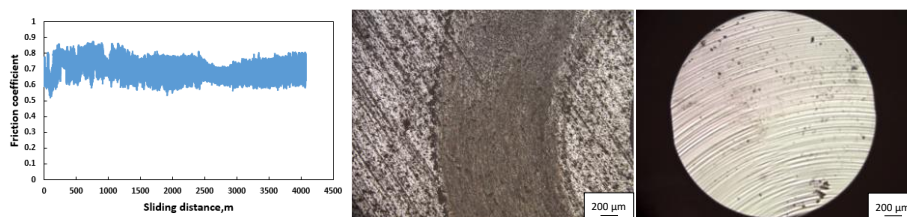
Fig.3 Friction Test Results under High-Humidity Conditions and worn surface images
